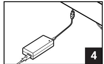
Unplug and re-plug in the Power Adapter to the Powered Recline Cable.
