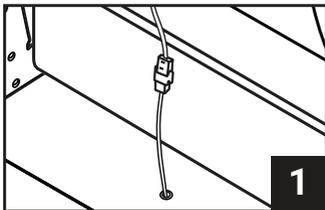
Unplug and re-plug the Powered Headrest Cables to each other.
