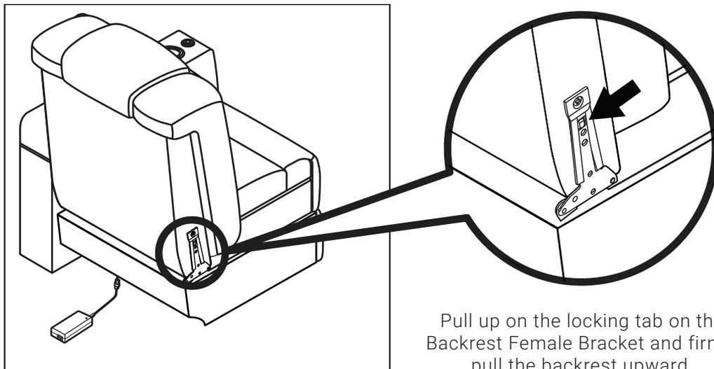
Pull up on the locking tab on the Backrest Female Bracket and firmly pull the backrest upward.
