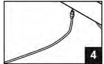
Unplug and re-plug in the Power Adapter Cable into the Seat Base Power Cable.
