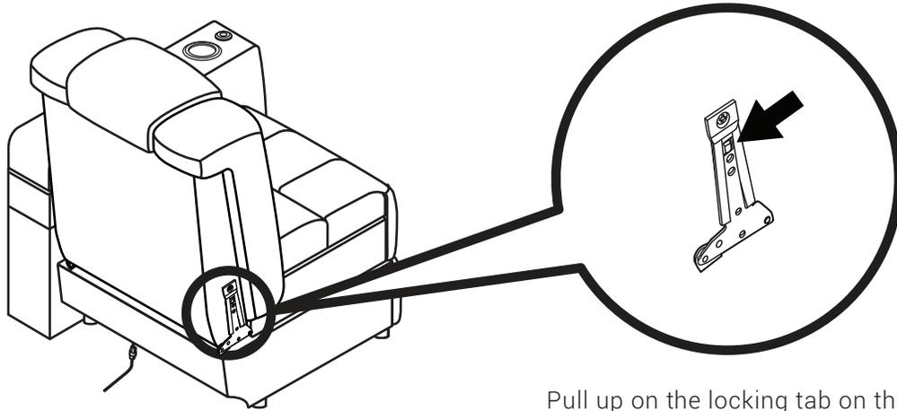
Pull up on the locking tab on the Backrest Female Bracket and firmly pull the backrest upward.
