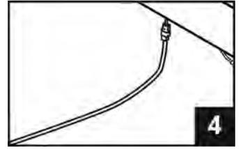
Unplug and re-plug in the Power Adapter Cable into the Seat Base Power Cable.
