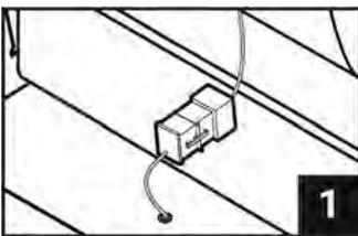
Unplug and re-plug the **Remote Cable Connection** to each other.
